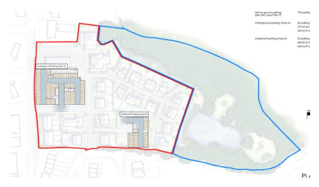
The above plan provides an indicative layout for the proposed underground and under-croft car parking. The above plan also shows relevant space for lifts and stairs access to the residential units above.
